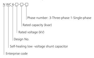
Note: The default rated frequency is 50Hz. For products with the rated frequency of 60Hz, mark 60Hz.
